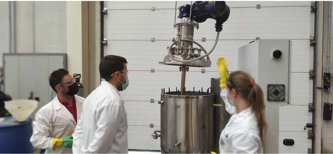
FIGURE 6. Scaling up of the chemical treatment of OTP fiber.
