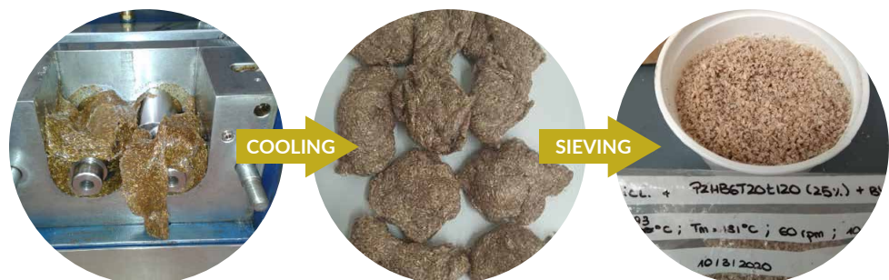
FIGURE 4. Manufacture of biocomposite at laboratory scale.
