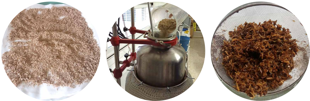
FIGURE 3. Shredded and sieved wood fiber from OTP waste (left), reaction configuration necessary to carry out chemical treatment of the fiber on a laboratory scale (center) and chemically treated OTP fiber (right).
